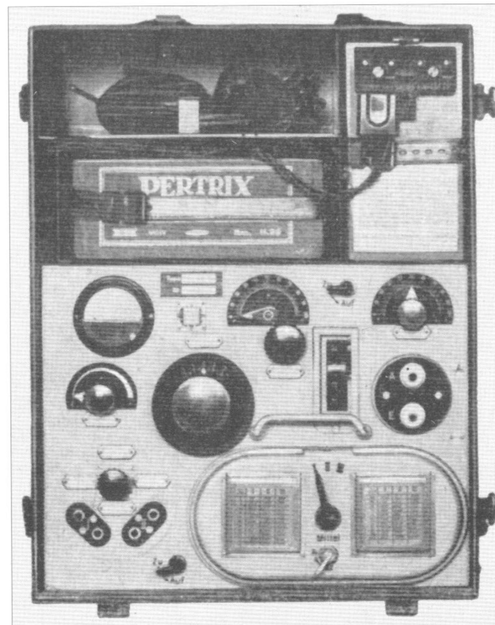
Left Fu 1 short-wave receiver of Torn.E.445 Bs type according to Wehrmacht standard of 1936. It was a 1st generation equipment with pin-socket electron tubes. In 1943 a new Fu 1 - Fu 25 standard was put to effect, which concerns common radio equipment of ground forces. Size: 46 x 36 x 22 cm.
