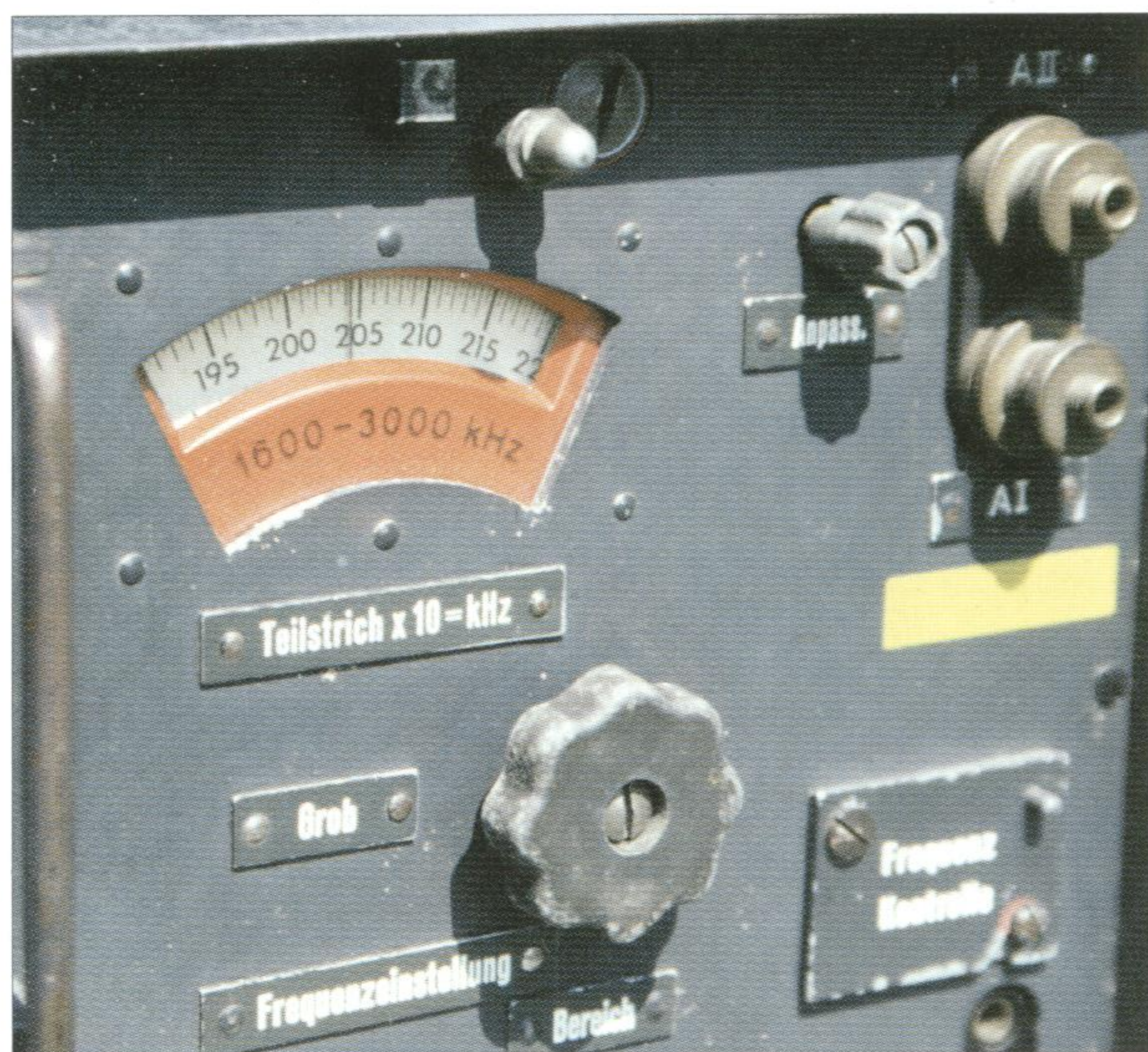
A top short-wave receiver earmarked for service with tank corps, was fitted to every commander's tank. Size 32 x 20 17 cm.
