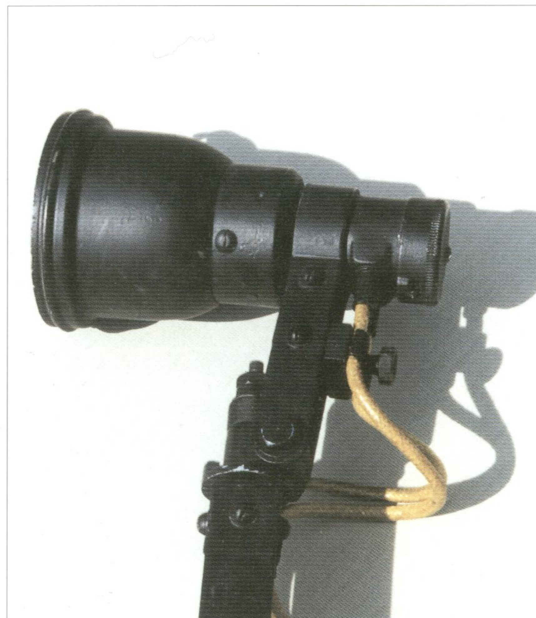
Various interior lights used in radio vans and aircraft. They were for 12 and 24V according to the type of vehicle.
