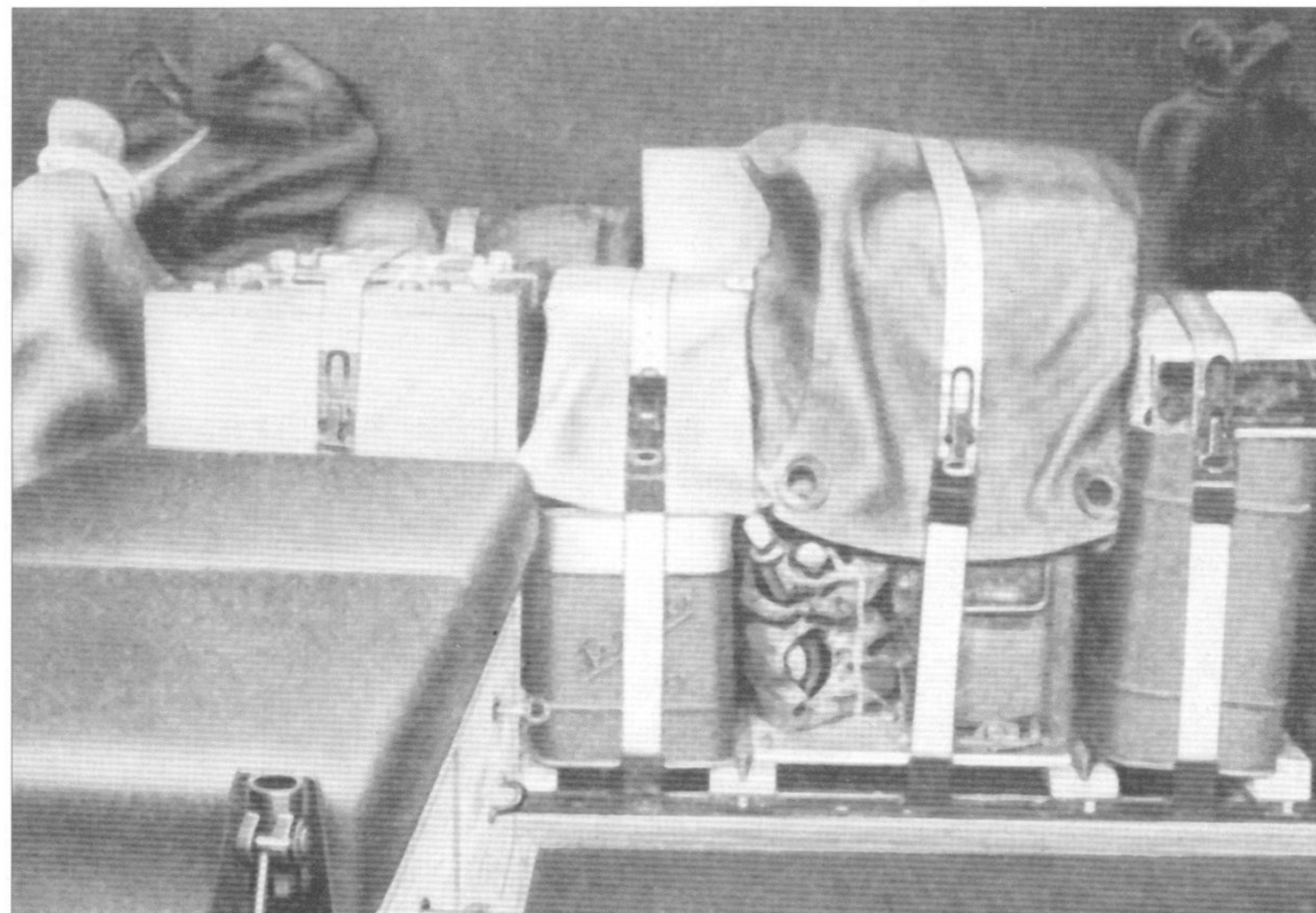
Left top a table for radios is placed. These versions still had the radios strapped to tables with webbing instead of rubber-block-mounted.
