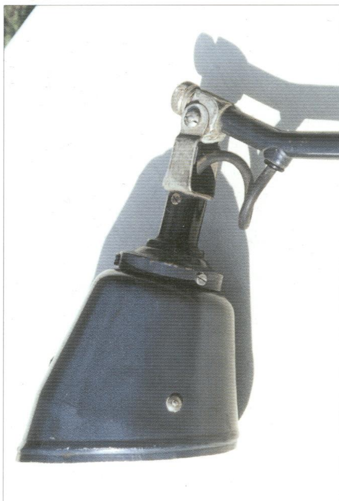
Various interior lights used in radio vans and aircraft. They were for 12 and 24V according to the type of vehicle.
