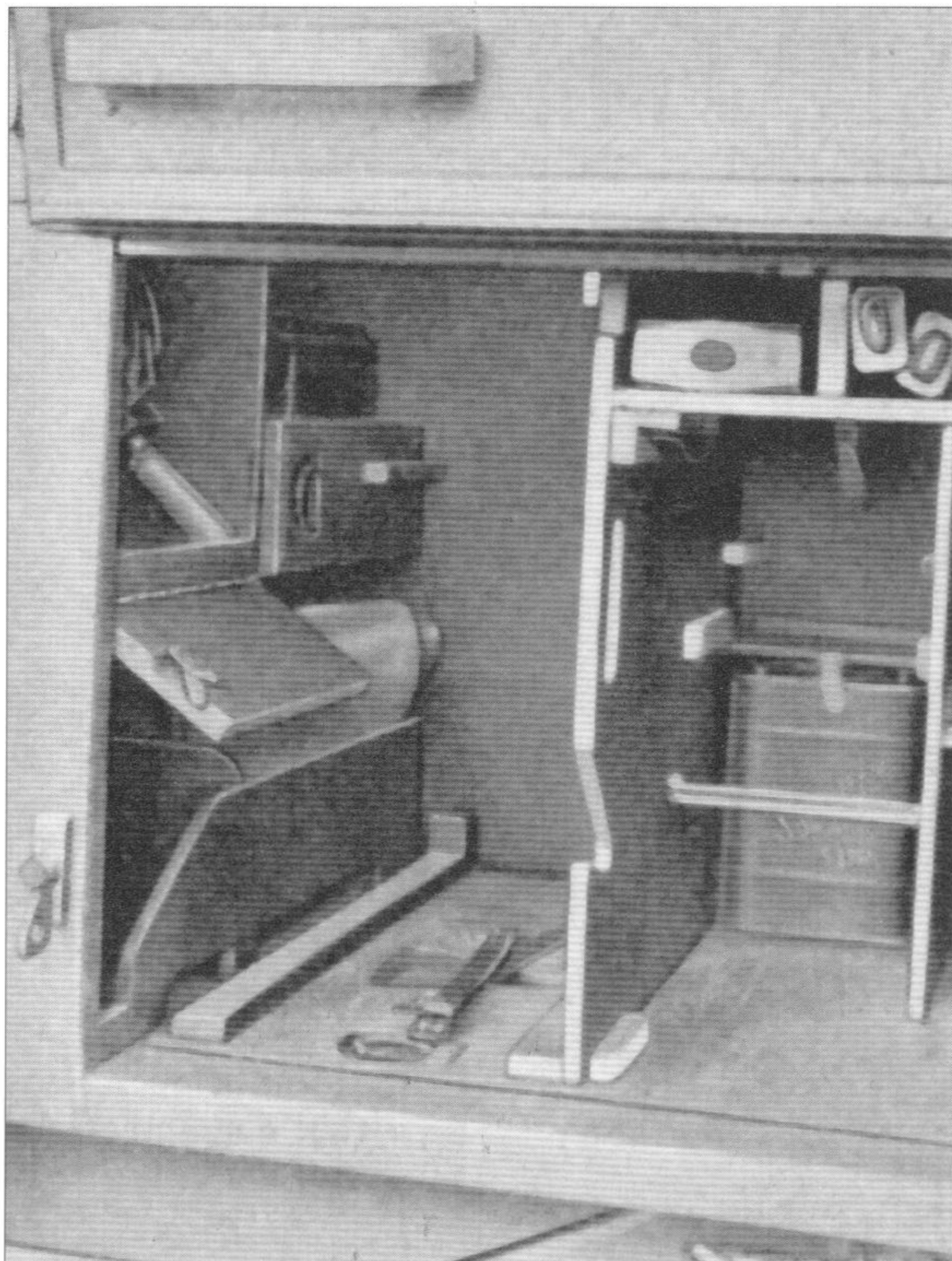
Fu 11 radio set. Unified Torn.E.b. receiver and 100 W.S. transmitter. Radio van provided for a communication of divisional headquarters with higher levels of command. Bottom an accessory box accessible from outside of the Kfz. 17 van.
