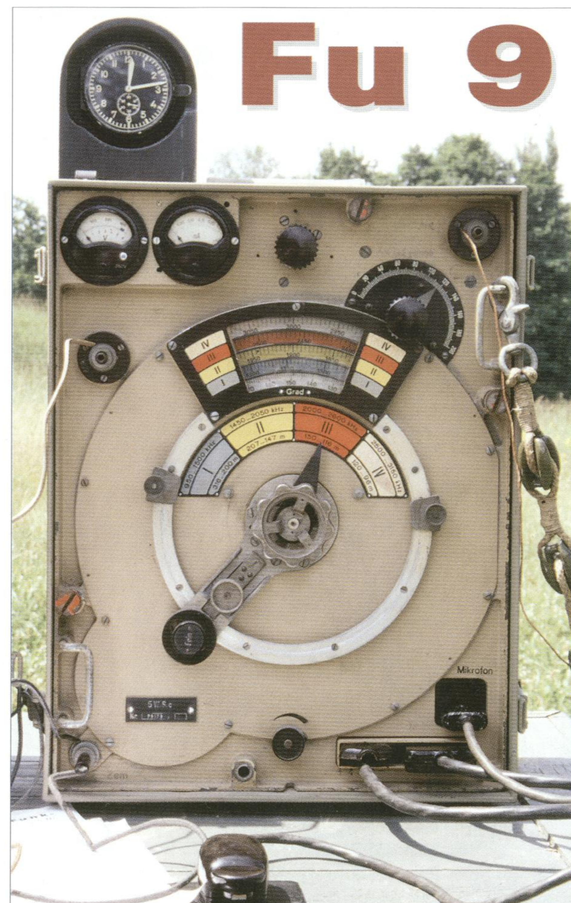
Fu 9 radio set: Torn.E.b. receiver, 5 W.S. transmitter, frequency range 0.95 - 3.15 MHz. Tactical use for communication between divisional and brigade level.
