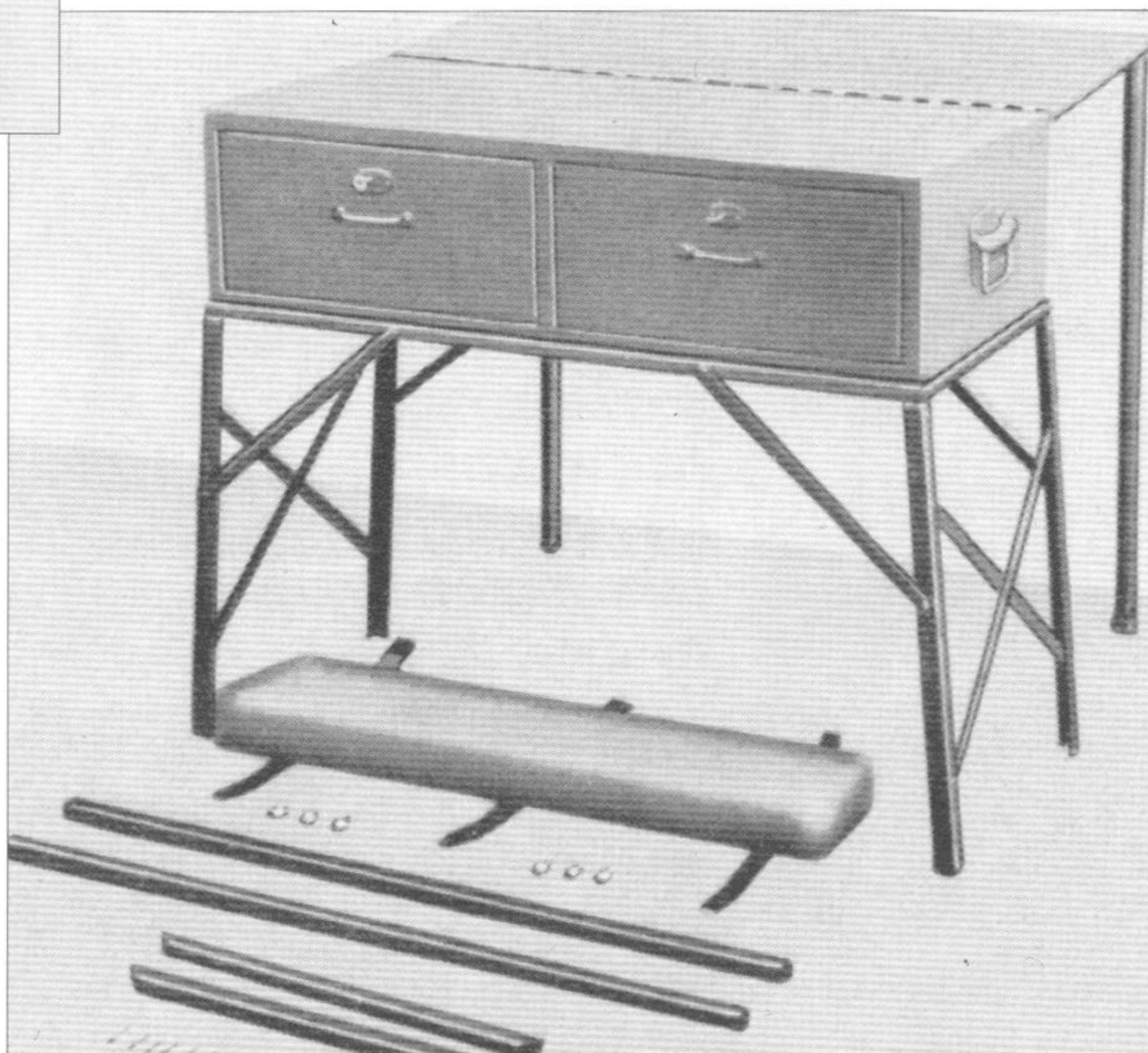
Bottom centre shows a frame holding the accumulator onto the vehicle floor, right with battery in place, left a detachable bench with storage space is shown.
