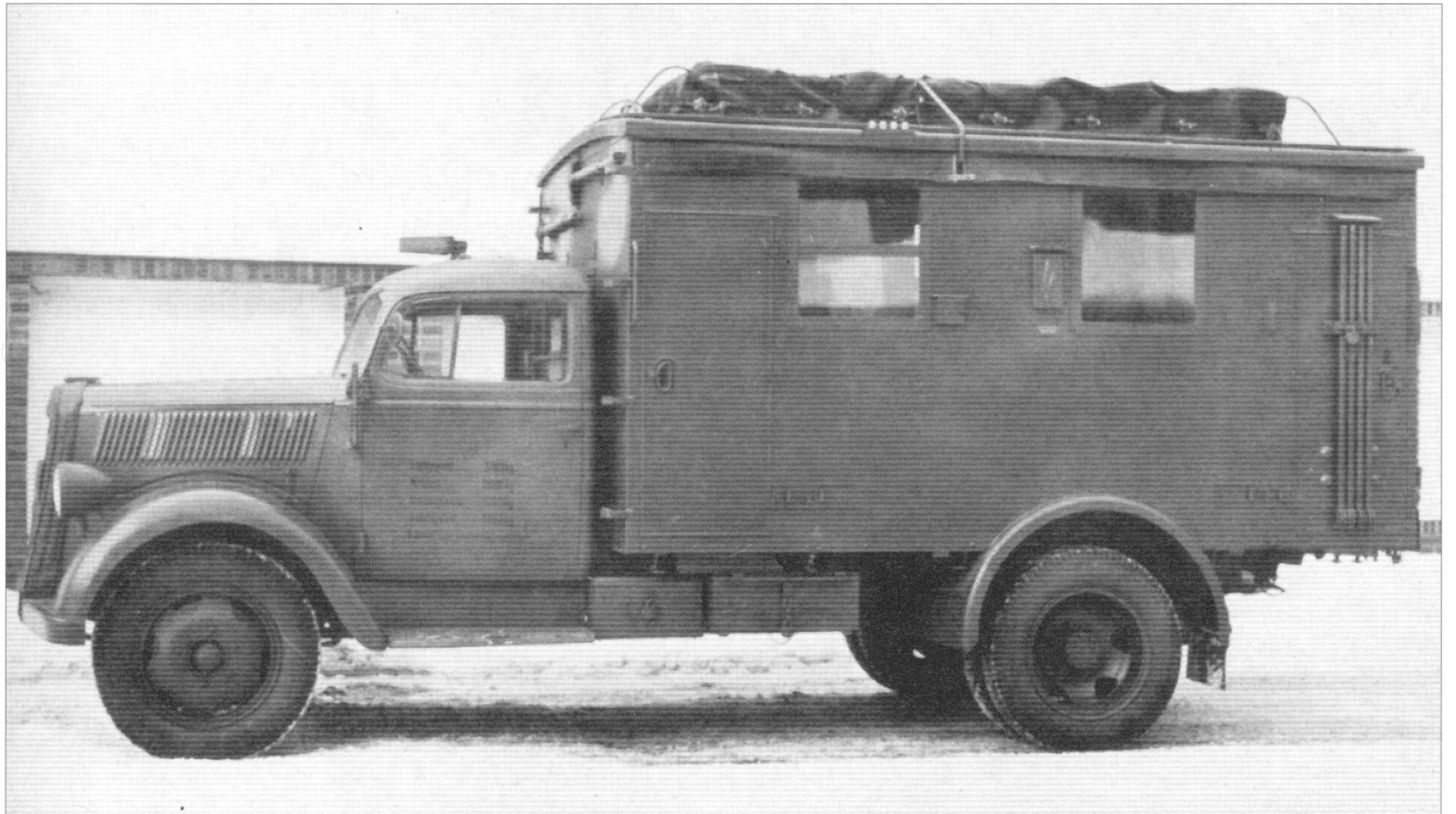
Opel Blitz Kfz. 305/22 receiving van. Note how the two telescopic antennae differ from the layout of version 18 depicted on opposite page.
