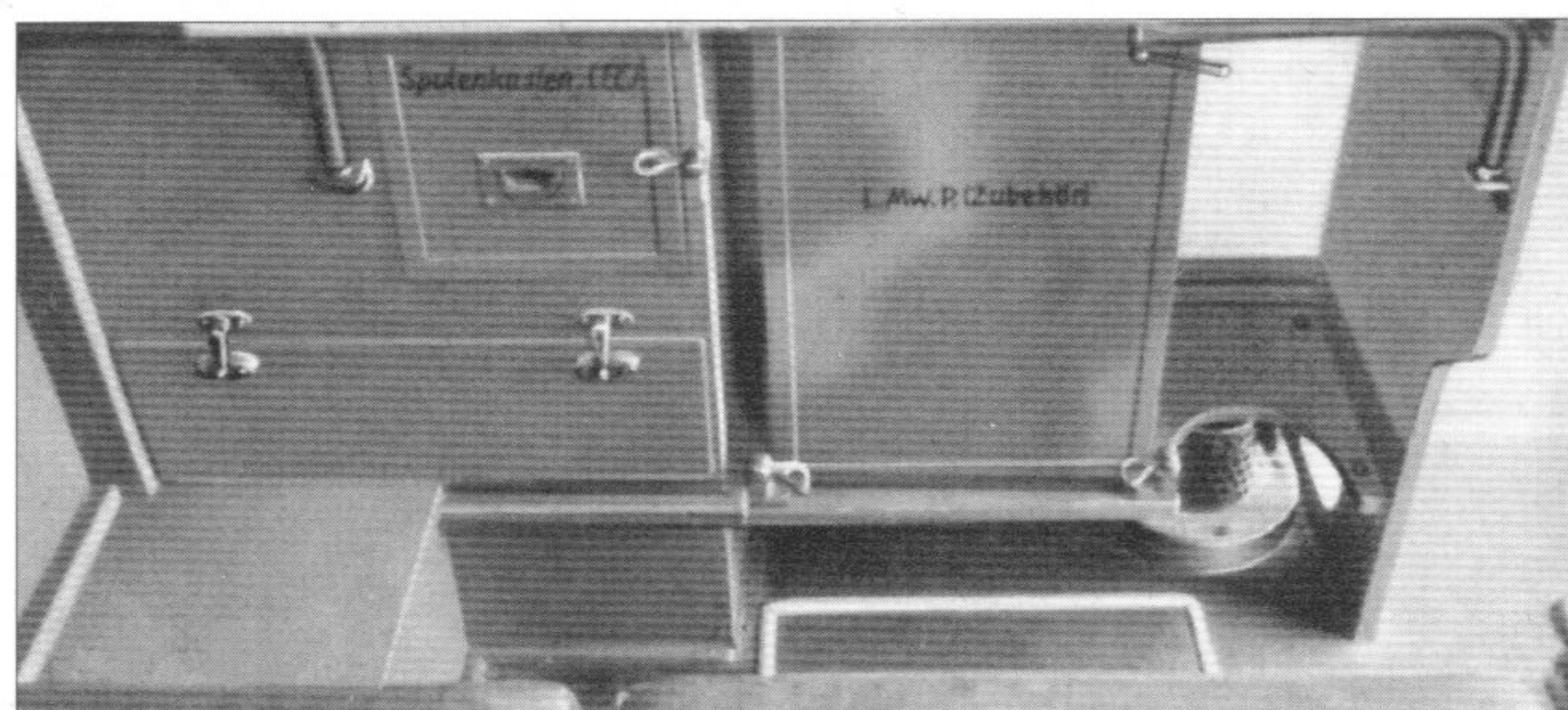
Pictures at the bottom of page show details of a radio van depicted on the opposite page. Above drawers with portable bobbins and two carbide lamps. Left bottom a drawer with jumpers, right a detail of a telescopic antennamast.
