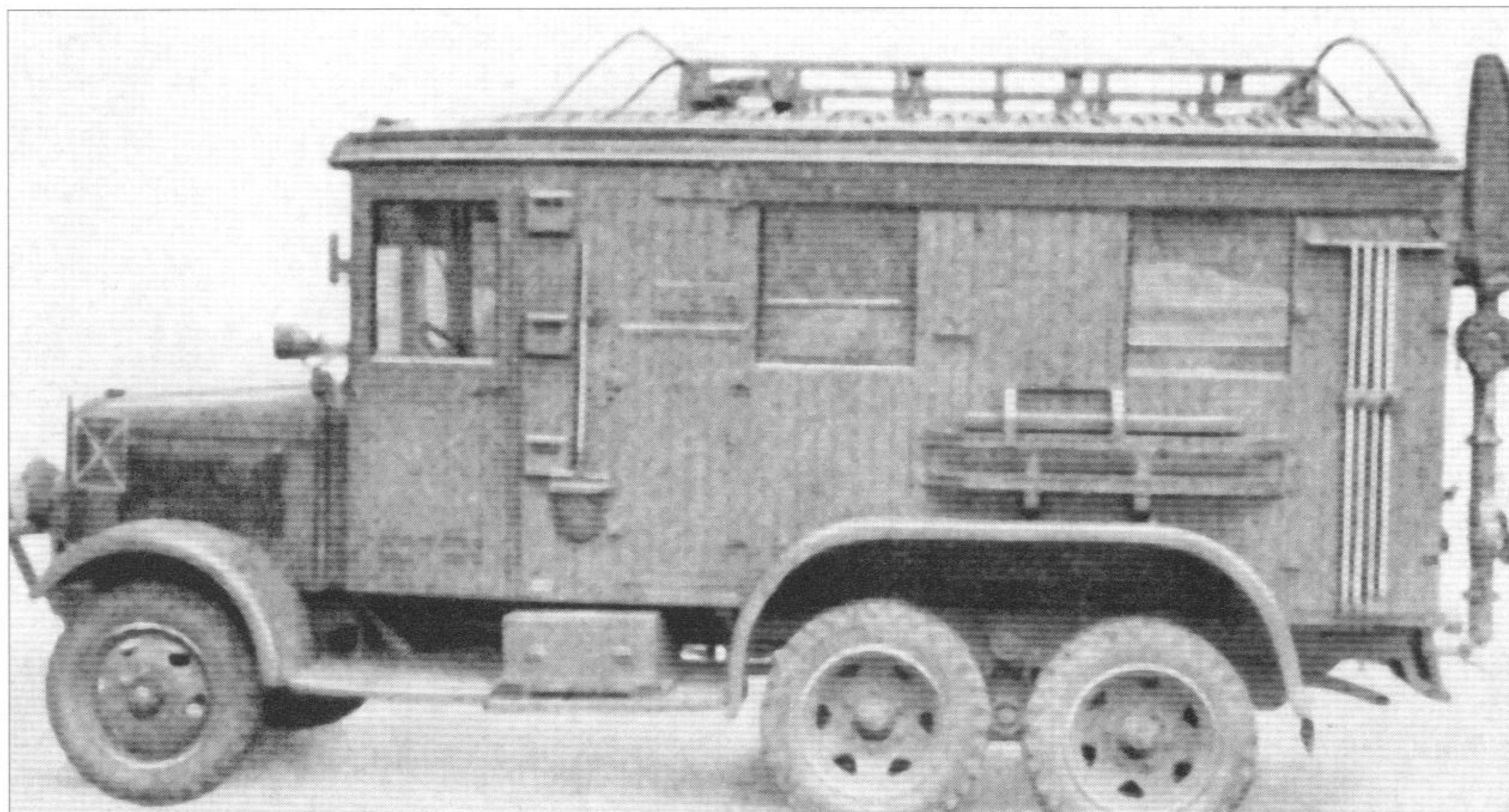
Bottom and right a radio van with 100 W.S. transmitter and Lw.E.a receiver.
