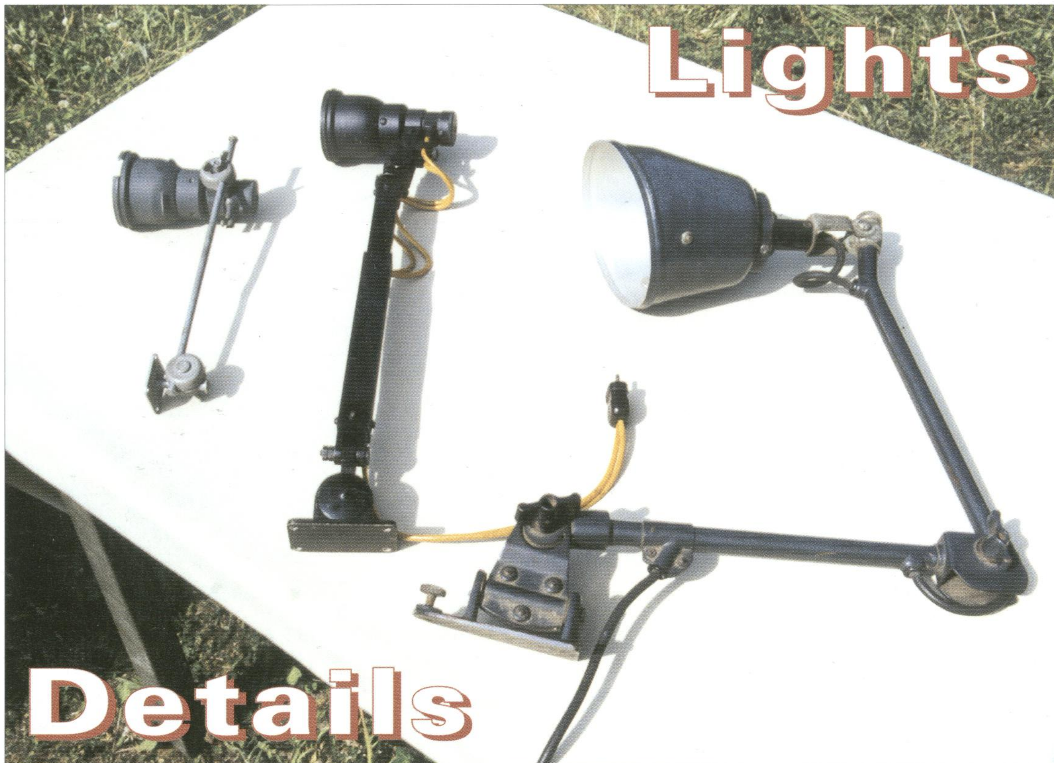
Various interior lights used in radio vans and aircraft. They were for 12 and 24V according to the type of vehicle.
